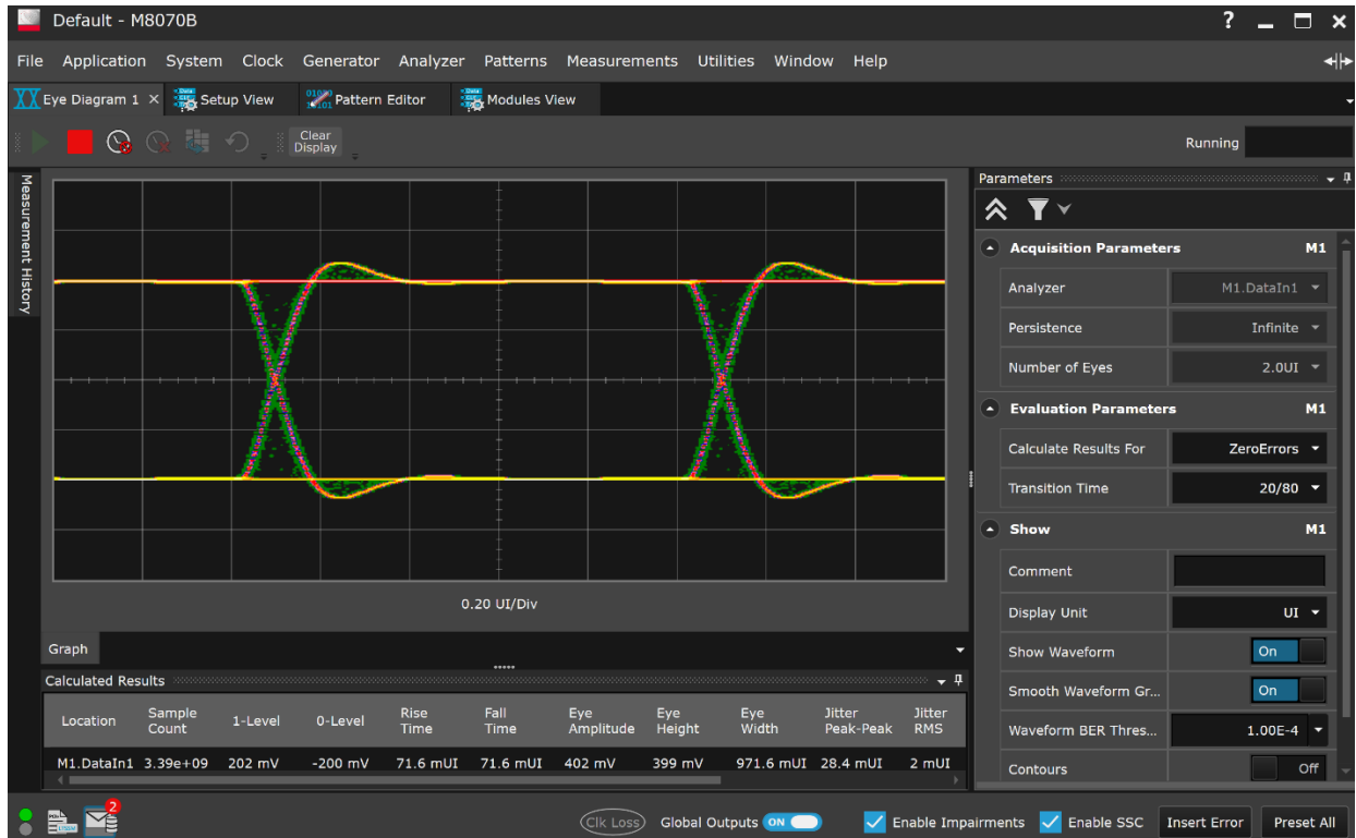
Figure 12. Eye diagram measurement with J-BERT M8020A Analyzer
